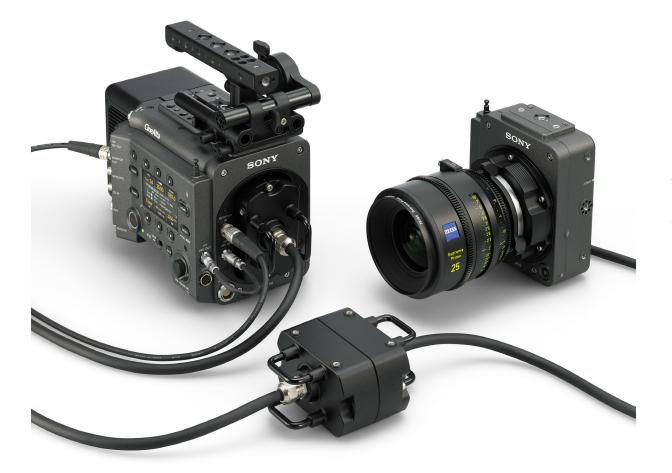
The VENICE camera body plate has a 24V DC input connector (Fischer 3pin). This makes it possible to provide 24V DC output at the camera head using a Fischer 3pin cable. When 12V DC output is required, the Hirose 4pin connector on the VENICE camera can be utilized by using Hirose 4pin to Fischer 3pin cable.
